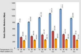
Fig. 3.20. Static elastic modulus of 6 AC types.
