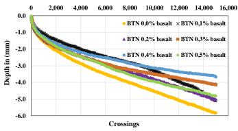
Fig. 3.4 Rutting depth results of the control and basalt fiber ACs.
