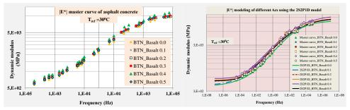
Fig. 3.29. |E\*| master curve of 6 ACs at reference temperature of 30°C.
