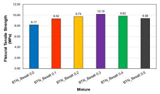
Fig. 3.7. Tensile strength results of different AC types with different fiber contents.
