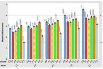
Fig. 2.16. Marshall flow (MF) results of all AC samples.
