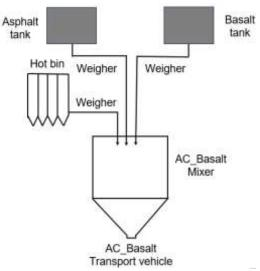
Fig. 4.7. Production of basalt fiber AC at the mixing plant
