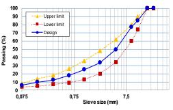
Fig. 2.2. Designed aggregate gradation curves.
