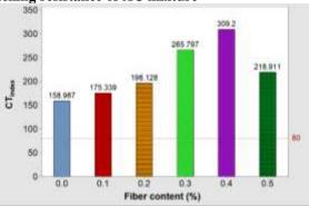
Fig. 3.14. CT<sub>Index</sub> results of different AC types with different fiber contents.
