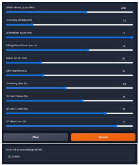
Fig. 4.4. GUI illustration to predict basalt fiber AC's MS.
